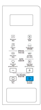
THIS FEATURE ALLOWS YOU to start the oven quickly. Press JET START button once, the oven starts to work at full power level. During cooking, press JET START to add time at 30 seconds interval. The longest cooking time is 90 minutes.
