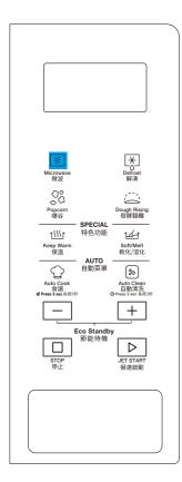
**То соок with** microwave power individually, press the Microwave button repeatly to select a cooking power level, then press +/- button to set a desired cooking time. The longest cooking time is 90 minutes.
