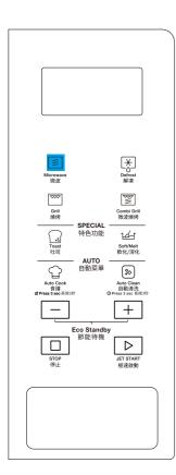
**Το cook with** microwave power individually, press the Microwave button repeatly to select a cooking power level, then press +/- button to set a desired cooking time. The longest cooking time is 90 minutes.
