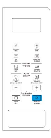
THIS FEATURE ALLOWS YOU to start the oven quickly. Press JET START button once, the oven starts to work at full power level. During cooking, press JET START to add time at 30 seconds interval. The longest cooking time is 90 minutes.
