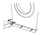
Container for the drained water: Place a low and wide container under the water filter in order to collect the residual water.
